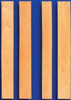
Tolerance on each face of two intergrown sound knots of 12 mm maximum diameter, or its equivalent, per linear meter.
