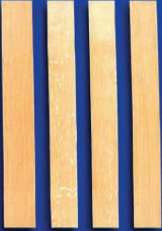
Straight-grained sawings, free from all deteriorations or sawing defect on all four faces.
