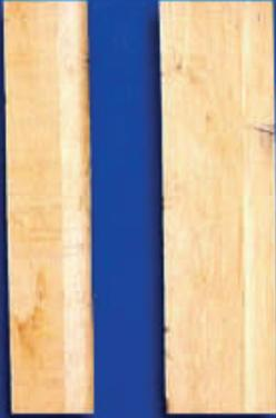
Sawn timber with sharp edges, no wane, with tolerance of small quantities of sound sapwood on two edges maximum, if it covers less than 15% of the width of the faces and the edges.
