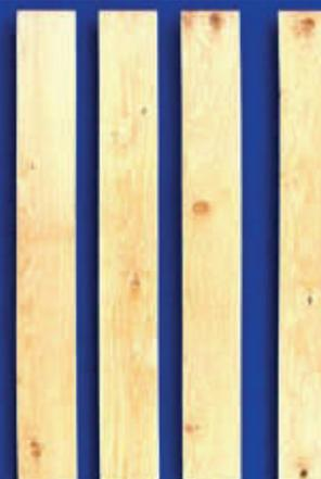
Presence on each face of small knots without limitation, and of a maximum of three sound knots per linear meter, maximum diameter not to exceed one half of the width of the timber or 40 mm or equivalent.
