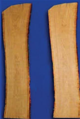
Boules in which two thirds of the boards are clean, straight, with little sapwood, grain practically straight, and with a regular heart.
