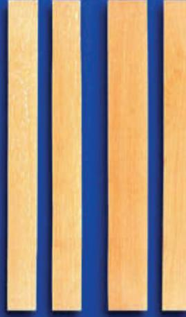
Straight-grained sawings, free from all deteriorations or sawing defect except for 20% of parts which can have one intergrown sound knot of 10 mm maximum diameter, or its equivalent, per linear meter on one face or one edge. If a piece is smaller than 1 m the entire piece will be accepted.
