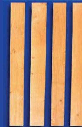
Presence on each face of small knots without limitation, and of a maximum of three sound knots per linear meter, maximum diameter not to exceed one third of the width of the timber or 25 mm or equivalent.
