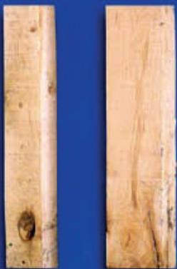
Sawn timber with tolerance of wane without limitation, leaving, on the faces and edges, a width of at least 60% of nominal.
