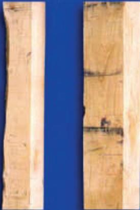
Sawn timber with sharp edges, no wane, with tolerance of small quantities of sound sapwood on two edges maximum if the minimum width exceeds 90% of the width of the piece.
