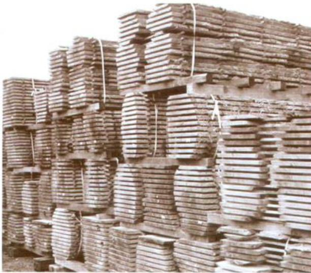
kilns. Timber is brought down to 12 to 14% moisture depending on thickness. EWT also has 15,000 sq ft of buildings for storing the kiln dried wood. The newest building is covered with solar panels which generate approximately 40K kilowatts a year, or about half of the electricity used by the company.
